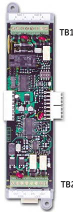
Signaling Line Circuit and NACs are supervised and power-limited.
